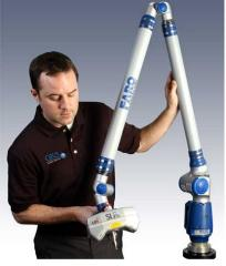
System scanning accuracy to +/-0.0020" (0.050mm) is attainable (system configuration-dependent ANSI B89 ball bar test). SLP laser probes come in three laser line lengths from 1.5" (33mm) to 10" (250mm).
